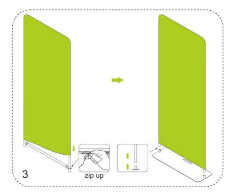
To wrap the fabric banner on the frame and zip up, afterwards install whole display stand to the base.
