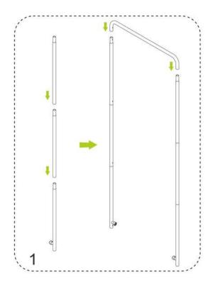
To connect all the aluminium tubes according to the numbering
